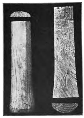
Fig. 40.—View of surface and interior of axe handle attacked by powder post borers. Note that few holes on surface do not indicate extent of damage to interior.
